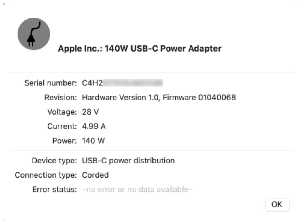
Figure 1.3: Example report for an Apple AC adapter. For power supplies with USB-C technology, the report also indicates the current charging mode as negotiated by the devices.
