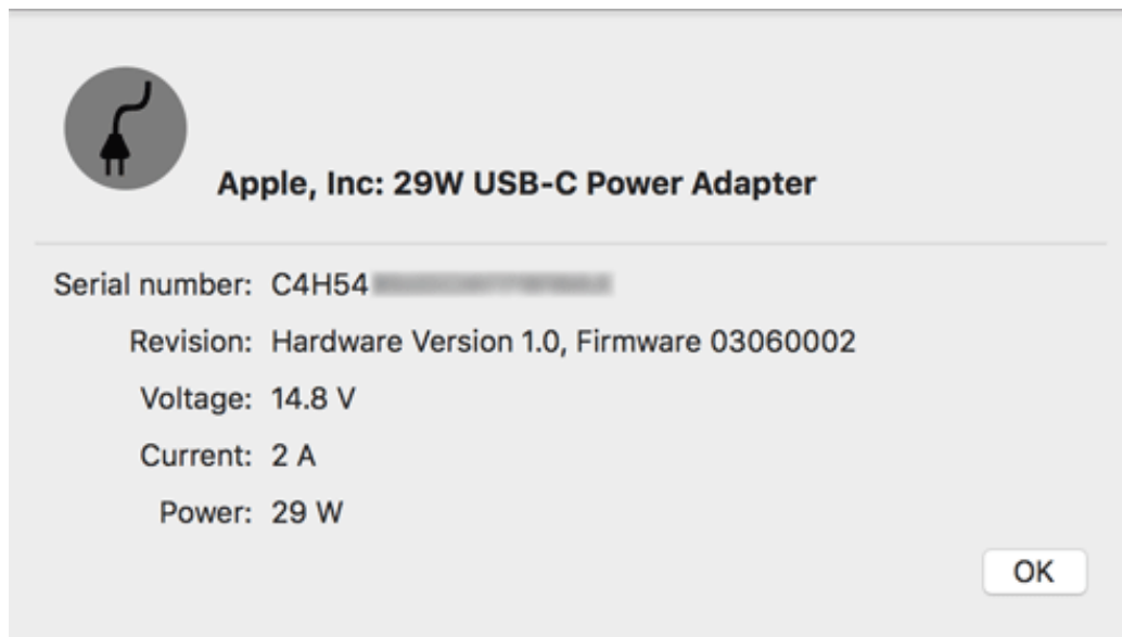
Figure 1.2: Example report for an Apple AC adapter. For power supplies with USB-C technology, the report also indicates the current charging mode as negotiated by the devices.
